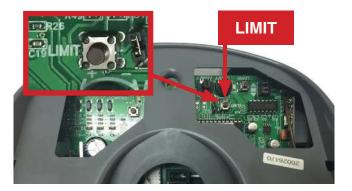
Press and hold the 'Limit' button for three seconds. The unit will beep three times to confirm the unit is in limit setting mode.
